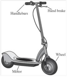
All transportation vehicles have sub-systems or parts that work together to make them go. The scooter on the left has a motor for PROPULSION,A handle bar for
