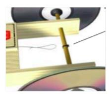
The loop you made will go over the **AXLE HOOK** and will spin the **AXLE.**
