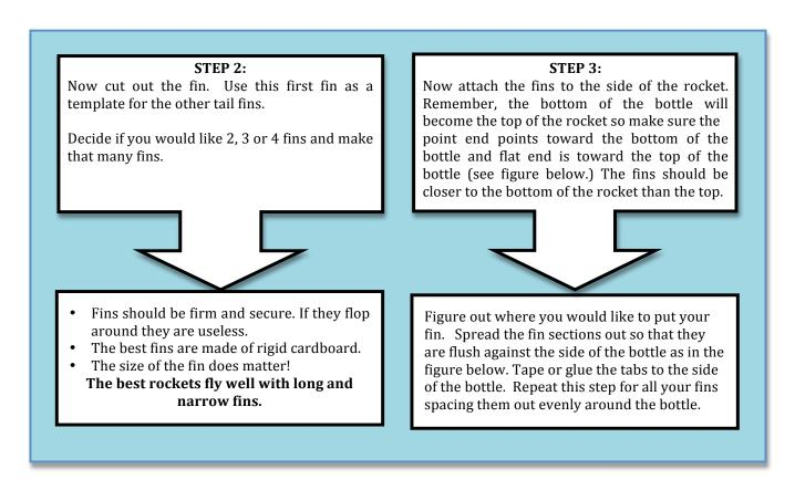
The fins need to be about 3 cm above the rocket's nozzle (the part of the bottle where the cap screws on).
