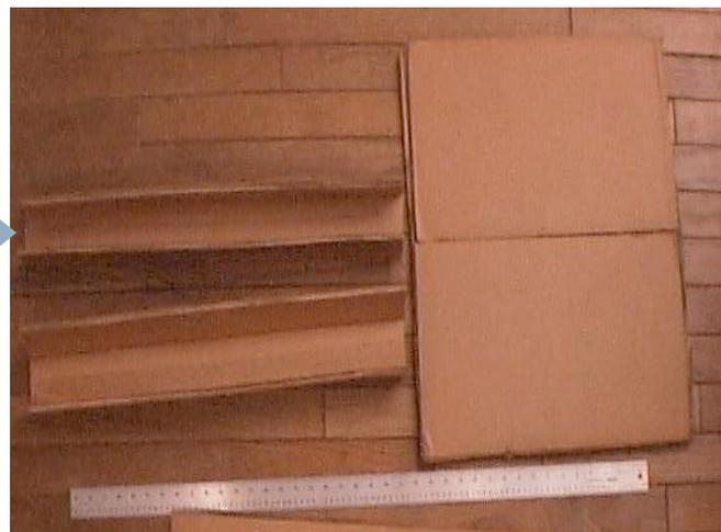
9. Fold the beams twice along their length to give a triangular cross section.
